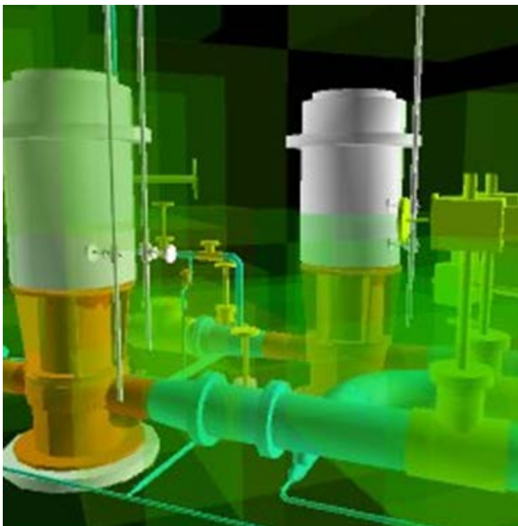
Fig. 2. Spatial distribution of dose rate around equipment and piping components
